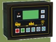
Operation of the module is via pushbutton controls mounted on the front panel with AUTO, MANUAL, STOP/RESET, FUNCTION, TEST and START pushbutton. The first two pushbuttons feature LED 'selected' indications. Further pushbuttons provide LCD DISPLAY SCROLL and SET functions.
